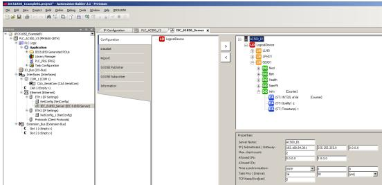
Create a dataset "Ping" and insert the GGIO1.ST\_IntIn.stVal c. IP-Configuration PLC\_AC500\_V3 R IEC\_61850\_Server X
