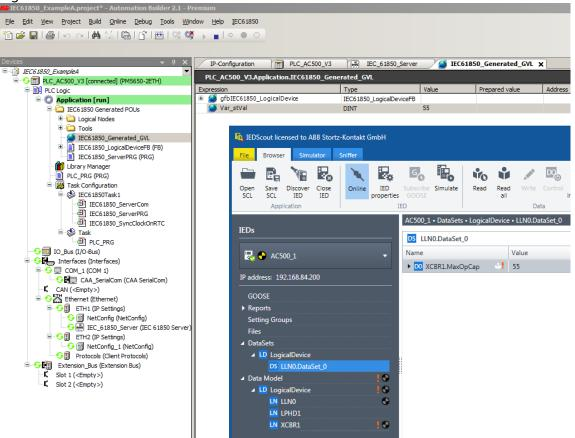
For an automatic update of the values the report can be enabled. Afterwards the AC500 actively sends a report when the value has changed, e.g. from 55 to 66:
