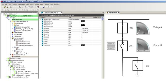
In the global variables the currents and voltages of all 3 phases are shown. Furthermore the positions of Disconnector (DC), Circuit Breaker (CB) and Earthing Switch (ES) can be monitored: 2 is open, 1 is closed, 0 is intermediate state.
