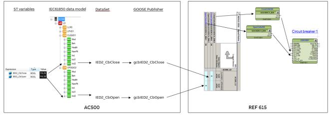
On AC500 side the signals are mapped to IEC 61850 data model (Logical Node GGIO, Data object Ind), packed into datasets and sent as Goose control blocks.
